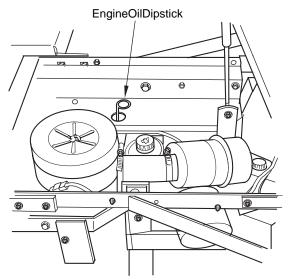
Figure 7-4 Engine Fill Stick
